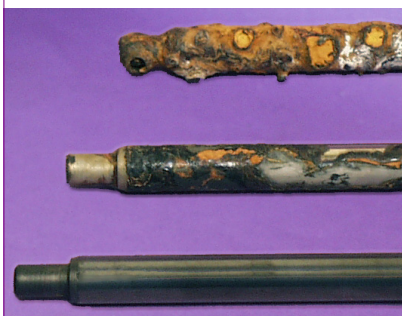
Gas Spring Rods after 560 hrs in salt spray (ASTM B117)
